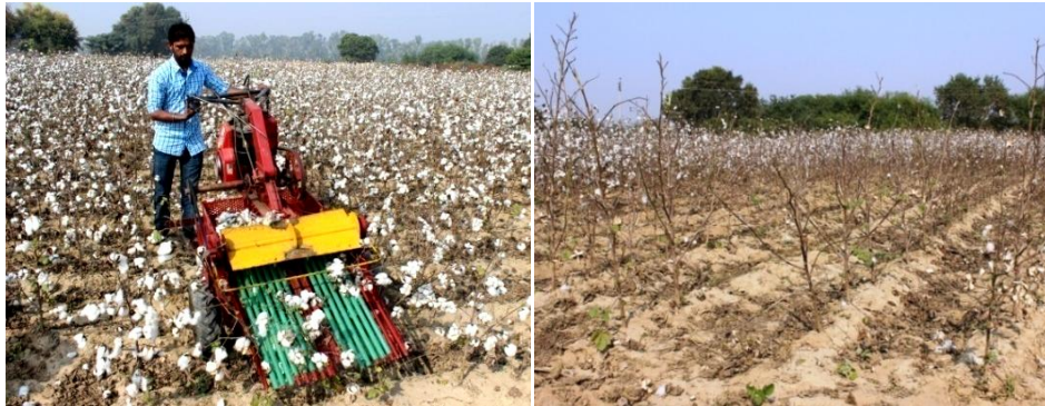
Figure 2. Operational view of cotton stripper in the field before and after harvesting of crop
