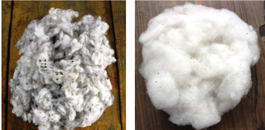
Figure 6. Cotton sample before and after trash analyzing operation
