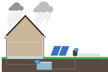
Figure 1. Combining the rainwater harvesting with solar irrigation
