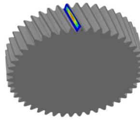
Figure 9. Contact stress on gear
