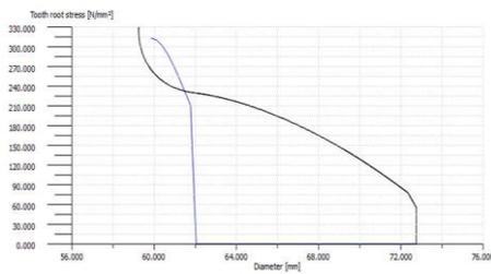
Figure 10. Graphical representation of tooth root stress on pinion
