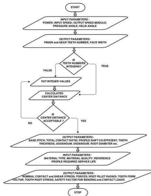
Figure 2. Flow chart for gear design in Visual Basic
