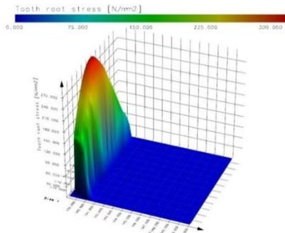
Figure 13. 3-D view of tooth root stress on gear
