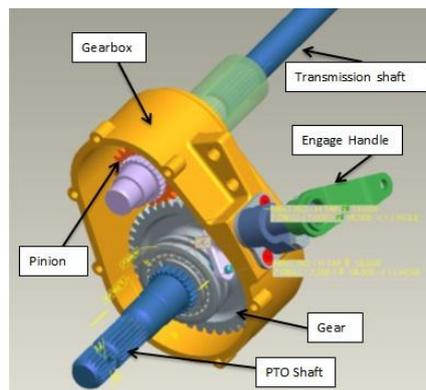
Figure 1. Pro-e model of front PTO
