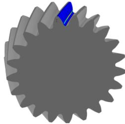
Figure 8. Tooth root stress on pinion
