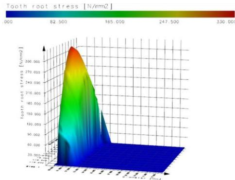
Figure 12. 3-D view of tooth root stress on pinion
