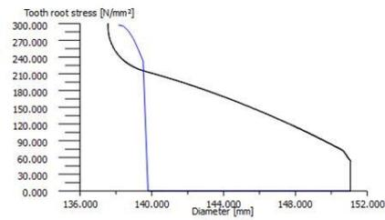
Figure 11. Graphical representation of tooth root stress on gear
