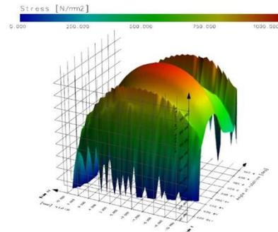
Figure 14. 3-D view of contact stress on gear
