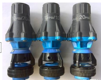
Figure 2. Fixed spray pressure heads used
