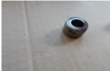
Slika 15. Oštećena rolnica koja usmerava kretanje šipke podizača šestog izduvnog ventila motora drobilice Figure 15. The damaged roll directing the chalk rod lift of the sixth exhaust crusher engine of a wood shredder
