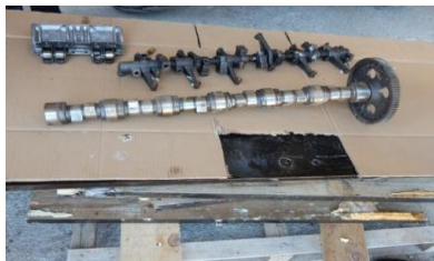
Slika 3. Bregasta osovina, osovina klackalica sa klackalicama i nosač rolnica motora Caterpillar tip 3126 -celokupan izgled Figure 3. Camshaft, rocker arm with swingarms and Caterpillar 3126 engine roller bearing - overall layout
