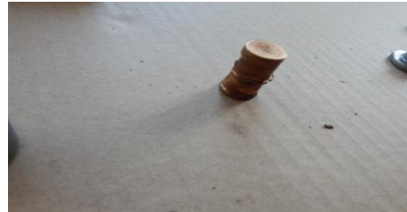
Slika 16. Oštećena osovinica rolnice koja usmerava kretanje šipke podizača šestog izduvnog ventila motora drobilice za drvo Figure 16. A damaged roll axis that directs the chalk rod lift of the sixth exhaust crusher engine of a wood shredder
