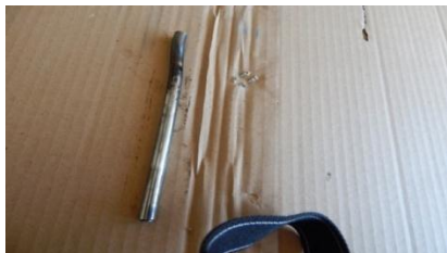
Slika 17. Oštećeno – polomljeno stablo (obostrano) izduvnog ventila na šestom cilindru pogonskog motora Figure 17. Damage view - broken on both sides of the exhaust valve tree on the sixth cylinder of the drive engine
