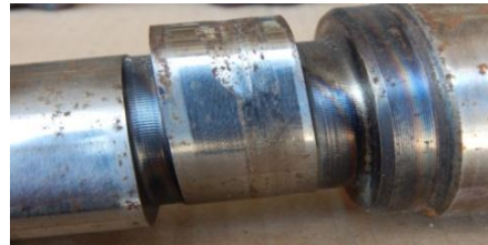
Slika 6. Bregasta osovina motora Caterpillar 3126- oštećenje brega šestog izduvnog ventila-pogled odozgo Figure 6. Caterpillar 3126 Camshaft - Six Exhaust Valve Camshaft Damage - Top View
