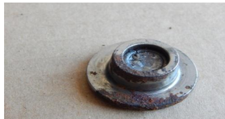
Slika 18. Oštećen - polomljen deo stabla izduvnog ventila na šestom cilindru sa svojim osiguračem u svom repnom delu pogonskog motora Figure 18. A damaged - broken part of the exhaust valve tree on the sixth cylinder with its fuse in its tail section of the drive engine
