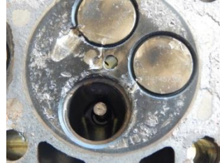
Slika 14. Oštećena glava motora, oštećeno sedište ventila i polomljen izduvni ventil na šestom cilindru motora Figure 14. View of damaged engine head, damaged valve seat and broken exhaust valve on sixth engine cylinder
