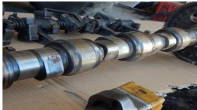
Slika 5. Bregasta osovina pogonskog motora Caterpillar tip 3126 Figure 5. Caterpillar 3126 Camshaft - Overall
