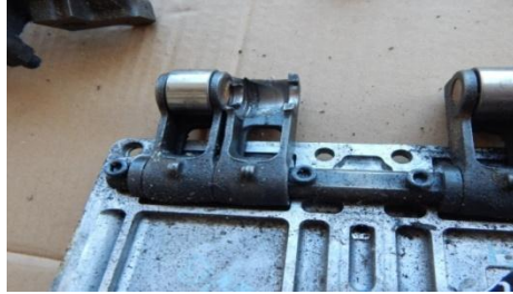
Slika 13. Oštećeno ležište rolnice koja usmerava kretanje šipke podizača šestog izduvnog ventila motora Figure 13. A damaged roll bearing that directs the choke of the sixth exhaust valve of the engine
