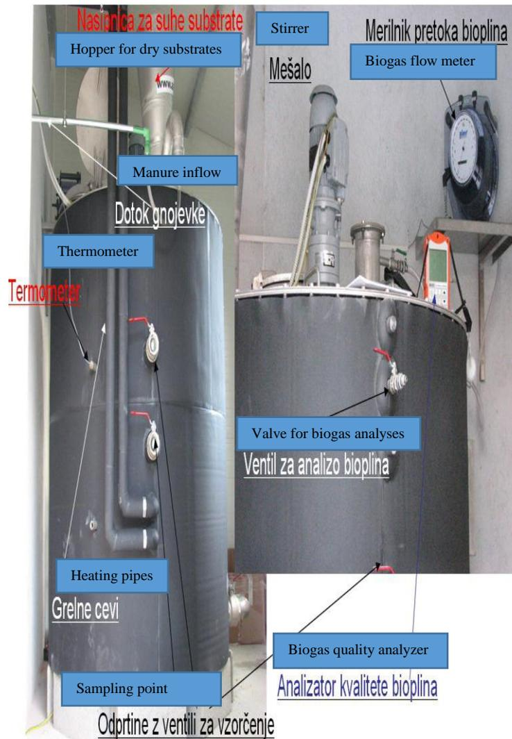
Figure 2. Experimental reactor
