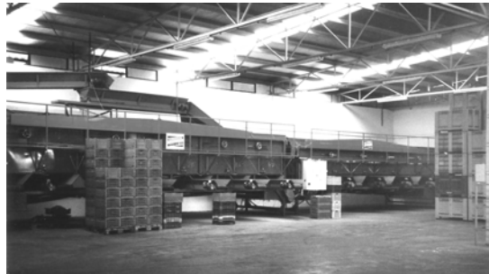
Figure 4: Stringed cucumber grading line type FLEISCHMANN
