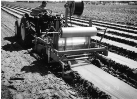
Figure 1: Ridge forming and foil laying machine type AF1
