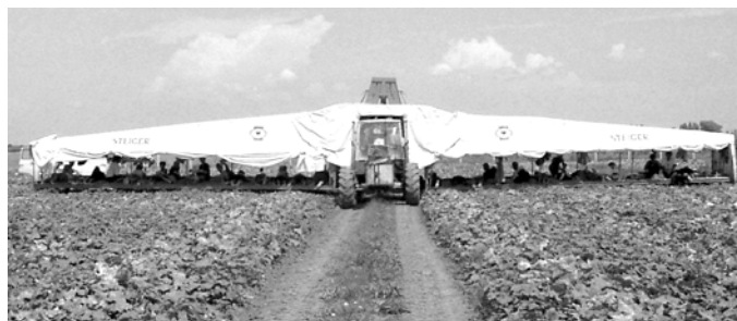
Figure 3: Belt cucumber picking carriage type STEIGER
