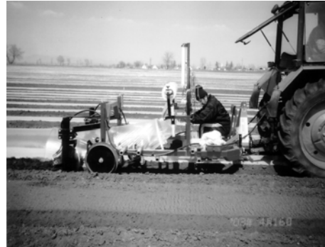
Figure 2: Tunnel-foil laying machine type AFF-1000
