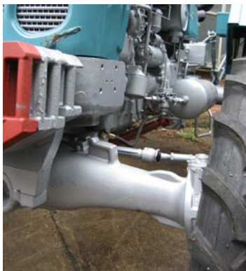
Slika 1. Novougrađeni pogonski most Figure 1. Newly installed drive axle
