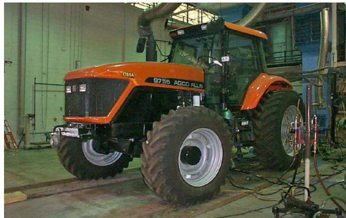
Figure 1. The tractor being tested on the PTO dynamometer The test apparatus in the foreground is measuring fuel flow.
