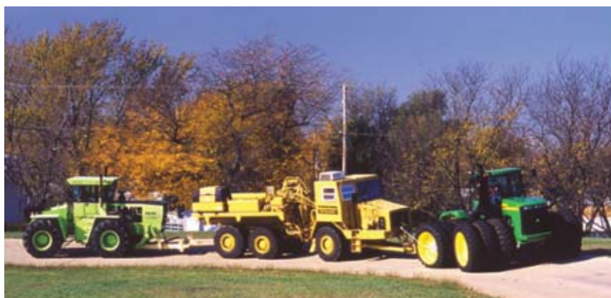
Figure 2. The lead tractor is being tested on the track during drawbar performance tests The two vehicles in tow are load units.
