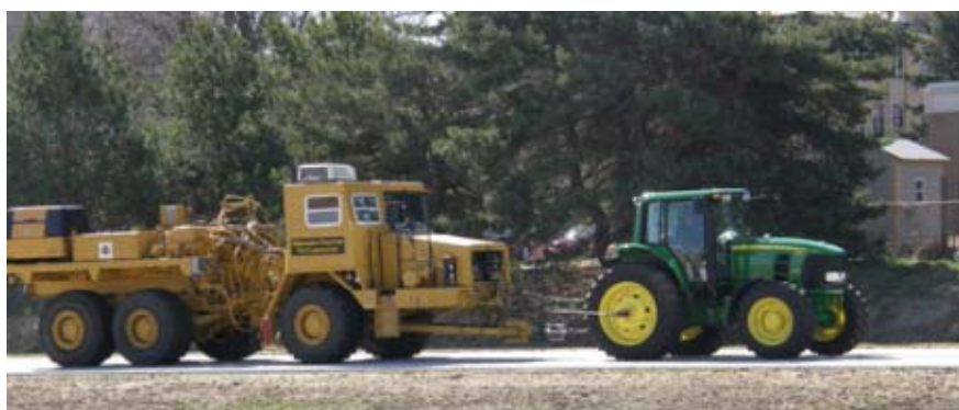
Figure 3. Tractor running on the test course Drawbar performance test being performed.
