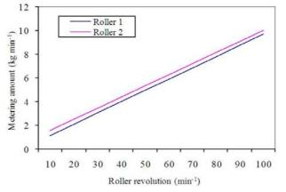
Figure 5. Composite fertilizer (20:20:0) metering function (Roller 1 and 2)
