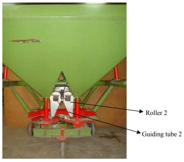
Figure 1. Rollers on spinner disc fertilizer applicator
