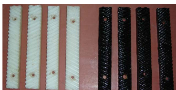
Figure 2. Comparison of nylon and cast iron rasp bars
