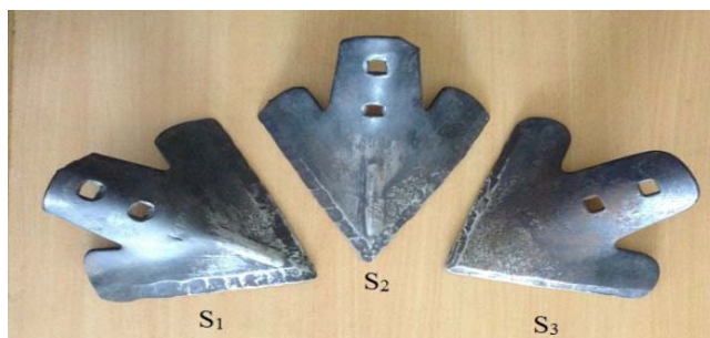
Figure 4. Different commercially available sweeps after operation in sand for 100 h
