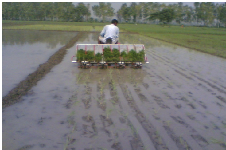
Figure 1. A view of transplanting by self propelled rice transplanter
