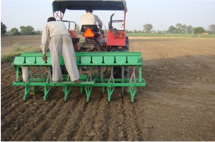
Figure 2. A view of paddy sowing by inclined plate type zero till seed-cum-ferti drill
