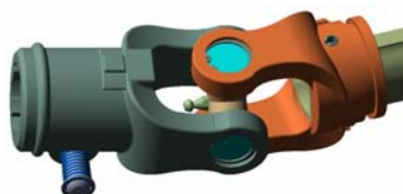
Slika 3. Kardanski zglob prikazan u 3D Figure 3. 3D image of a cardan joints
