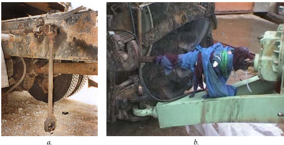
Slika 1. Primeri mogućih pojava opasnosti na dvostrukim kardanskim vratilima: a) oštećeno vratilo na kamionu sa cisternom i b) oštećeno vratilo na poljoprivrednom traktoru Figure 1. Examples of the possible occurrence of hazards on a double cardan shafts: a) the damaged shaft on a truck with tank and b) the damaged shaft on agricultural tractor
