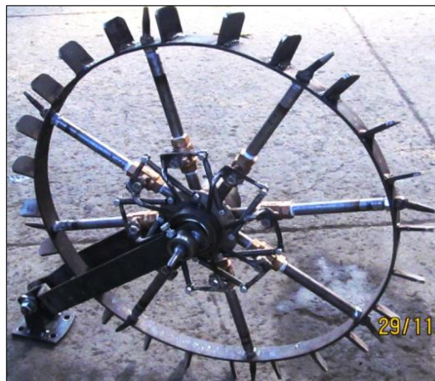
Figure 2. View of developed nitrogen (liquid urea) metering mechanism
