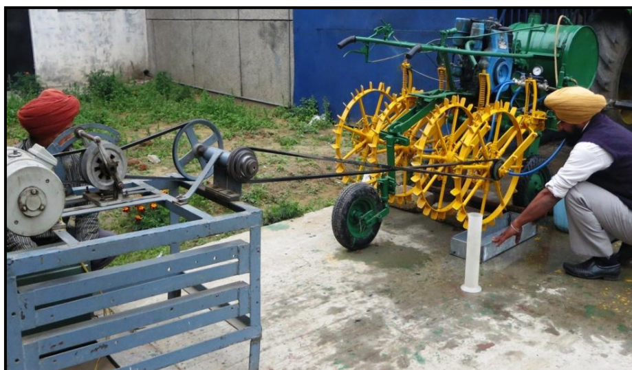
Figure 3. Laboratory evaluation of nitrogen (liquid urea) metering mechanism
