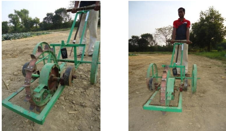
Figure 3. Figure of testing of braked wheel in field conditions
