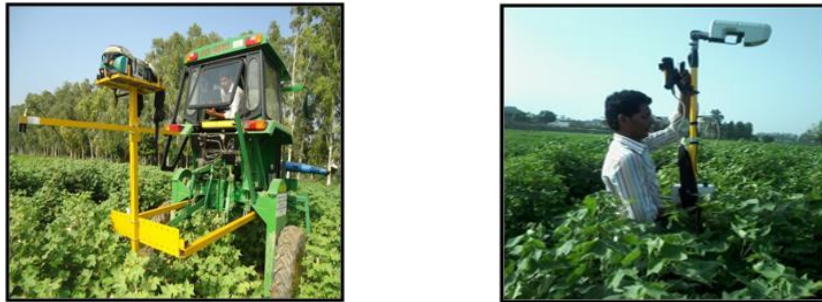
Figure 2. Capturing of spectral signatures of cotton crop using tractor mounted spectroradiometer and hand held GreenSeeker
