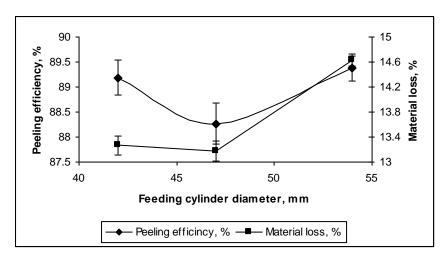
Figure 2. Effect of feeding cylinder diameter on peeling efficiency and material loss
