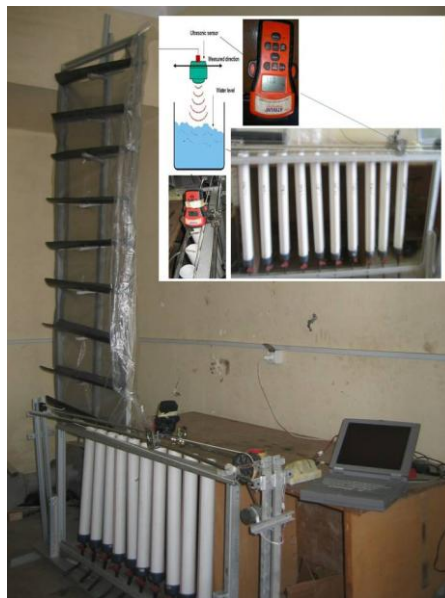
Figure 2. Development vertical patternator to measure the vertical uniformity for hydraulic sprayers
