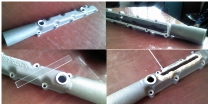
Slika 2. Adatacija usisne grane dizel motora Figure 2. Adaptation of the intake manifold of diesel engine
