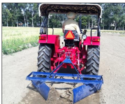
Figure 5. Operational view of bund maker in the field
