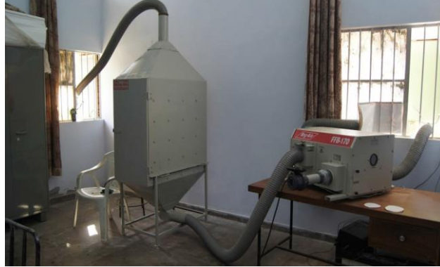
Figure 1. Desiccant based food dryer
