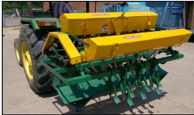
Figure 5. Developed raised bed inclined plate onion planter
