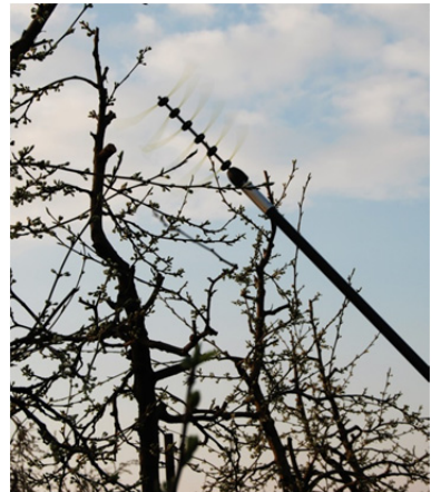
Figure 5. The Electroflor hand-held mechanical thinning device developed in France (Photo's: Frank Maas).
