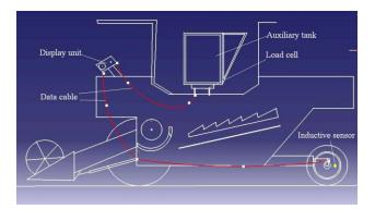
Figure 1. Design diagram of combine harvester installed with different components of indigenous yield monitor
