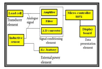
Figure 3. Block diagram of working of indigenous yield monitor
