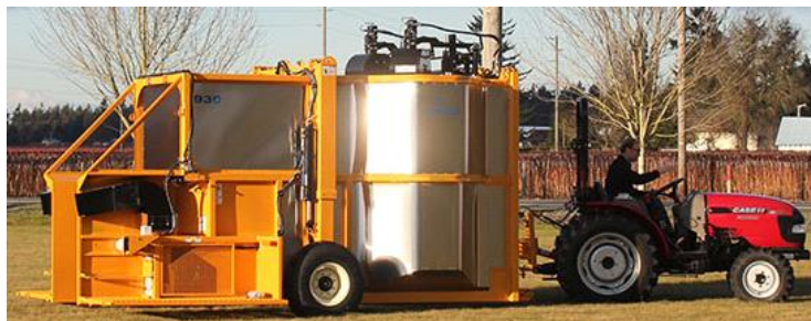
Slika 1. Vučeni berač jagodastog voća "Oxbo 930" [1] Figure 1. Trailed Berry Fruit Harvester "Oxbo 930" [1]
