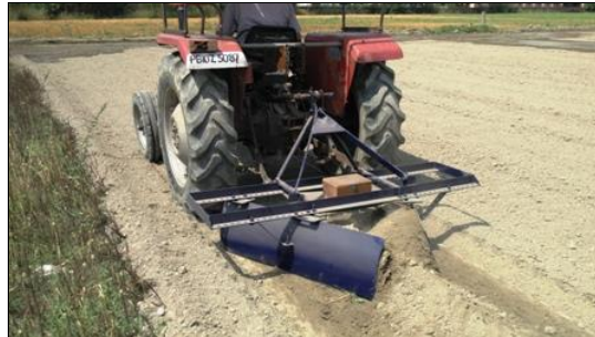
Figure 6. Developed soil pH measuring system mounted on a tractor operated bund former
