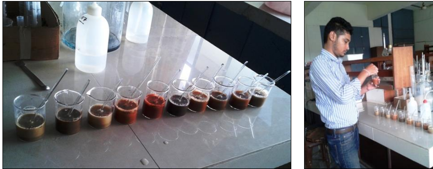
Figure 4. Soil samples collected from different locations and their pH measurement in laboratory
