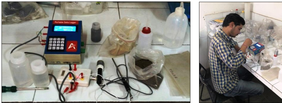
Figure 5. Calibration of pH sensor with data logger using collected soil samples
