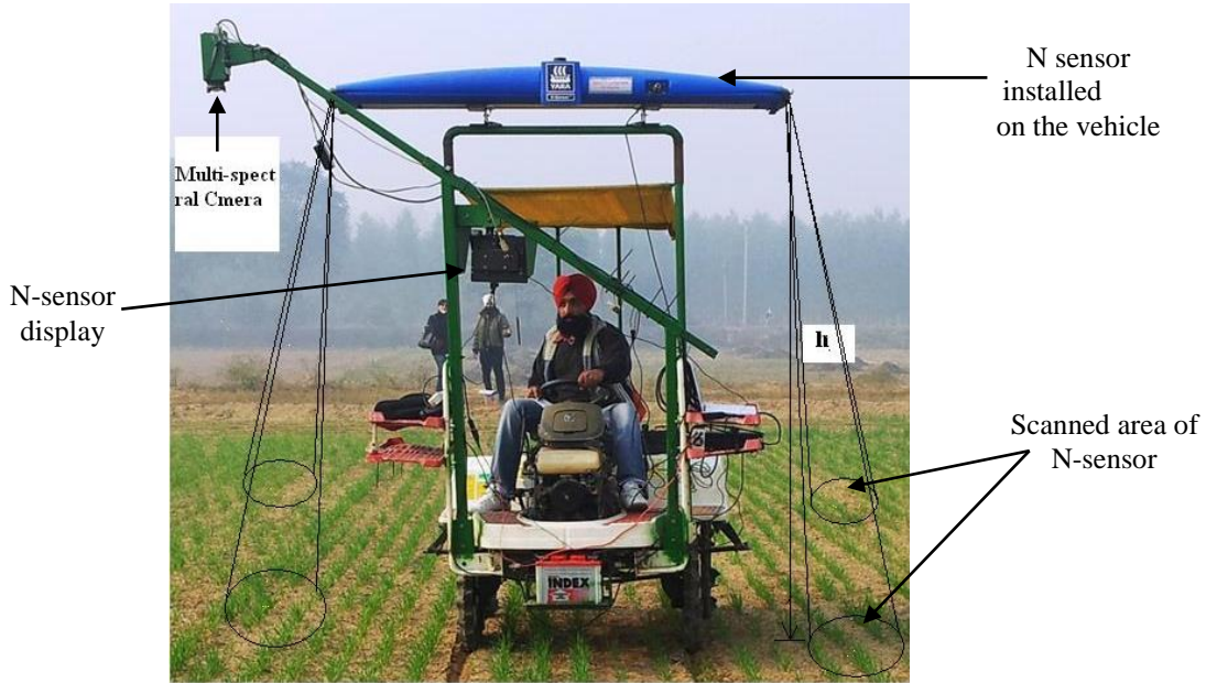
Figure 3. View of developed vehicle with installed sensor working in the field
