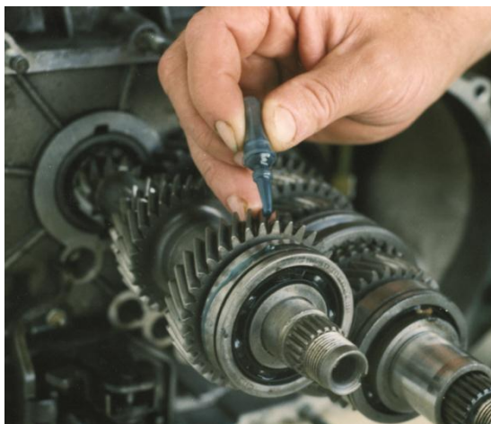
Figure 2. Restoration of rolling bearing fit
