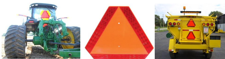
Figure 4. Slow Mowing Vehicle (SMV) sign for agriculture and forestry vehicles in Slovenia public traffic [18], [20].
