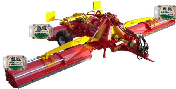
Figure 1: The position of the vibration sensors on the working machines, actually on the flail mower machine [11].
