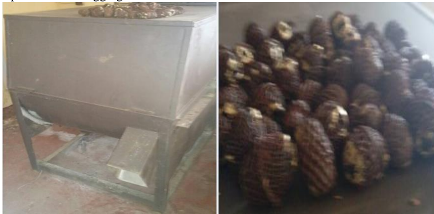
Plate 1: (a) Modified cassava attrition peeling machine
