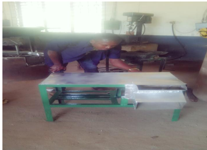
Figure 3. The Developed Plantain Chipping Machine
