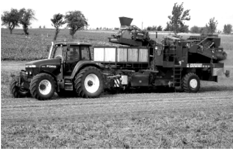
Fig. 1. Harvester Grimme SE 150 -60 with a device for filling and transferring the box (developed by Schoepstal Maschinenbau GmbH [7])
