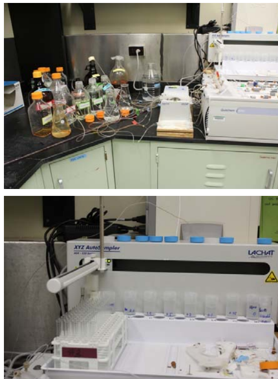
Figure 4. Quickchem 8500 analyzing system, all carrier solutions (up) and auto sampler of the system (down)
