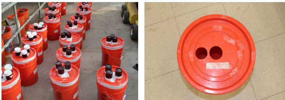
Figure 1. Five-gallon bucket with lid (two 5.1-cm holes were made on the lid)
