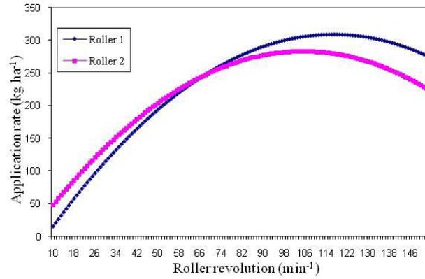
Figure 3. Dosage efficiency of rollers in 20:20:0 Composite application (kg ha<sup>-1</sup>)
