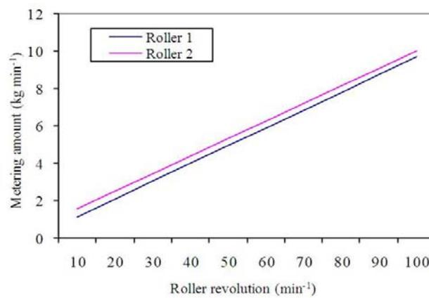
Figure 5. Composite fertilizer (20:20:0) metering function (Roller 1 and 2)
