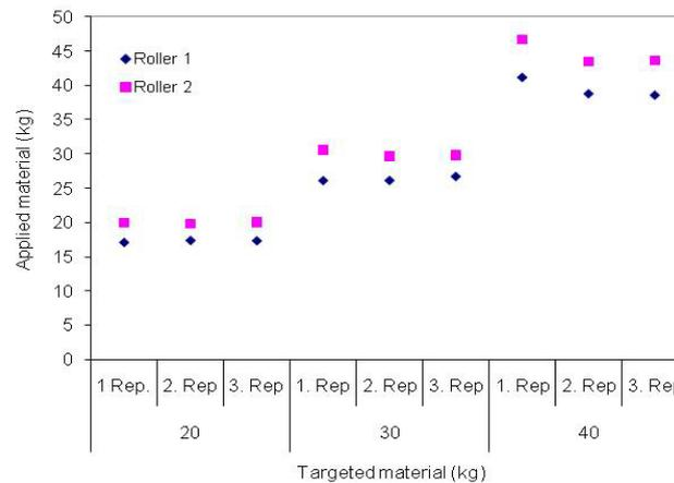
Figure 7. Composite dosage test (Roller 1 and 2)
