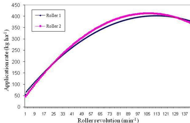
Figure 2. Dosage efficiency of rollers in 26% CAN application (kg ha<sup>-1</sup>)
