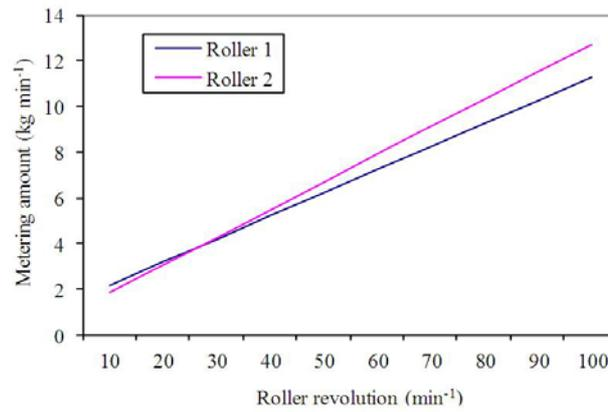
Figure 4. Calcium ammonium nitrate metering function (Roller 1 and 2)
