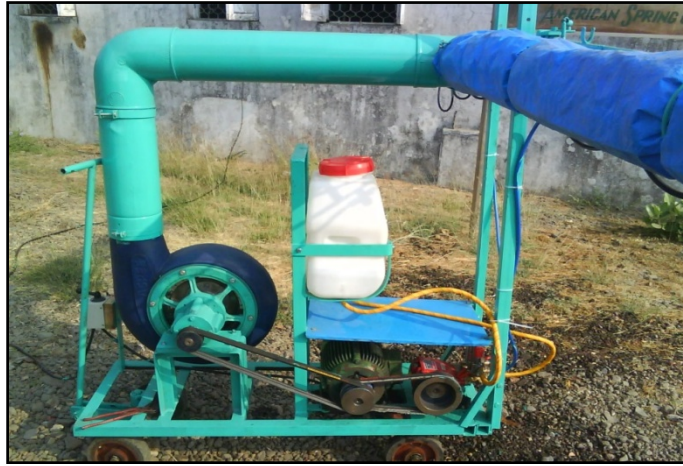
Figure 5. Side view of sprayer showing pesticide tank, blower, electric motor and pump
