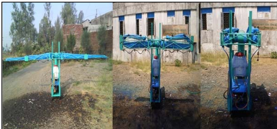
Figure 4. Front view of the air assisted sprayer showing the folding arrangement of the boom
