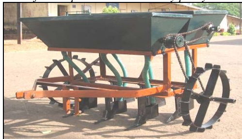
Figure 11. Developed bullock drawn dry paddy seed cum fertilizer drill
