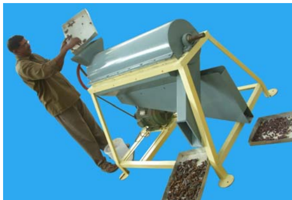
Figure 4. Tamarind deseeder (working condition)
