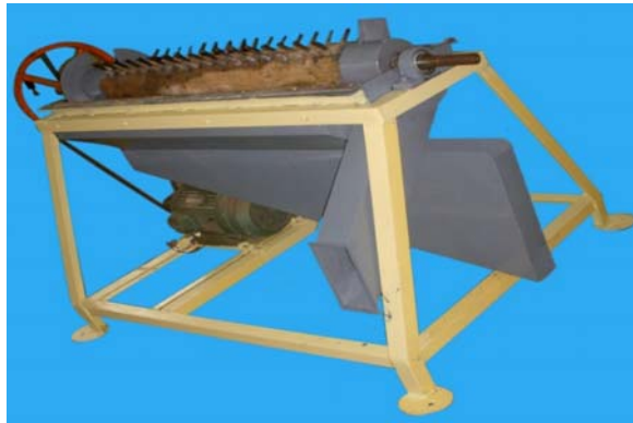
Figure 3. Tamarind deseeder (partly dismantled)
