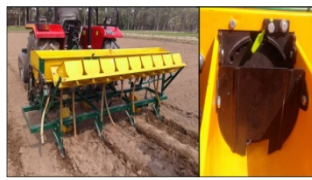
Figure 2. Inclined plate planter
