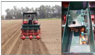
Figure 1. Raised bed maize multicrop planter
