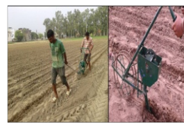
Figure 3. Manually operated planter
